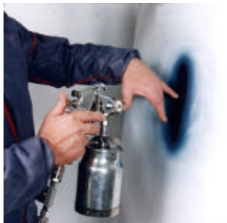
Figure 41.- Gun to Target distance
