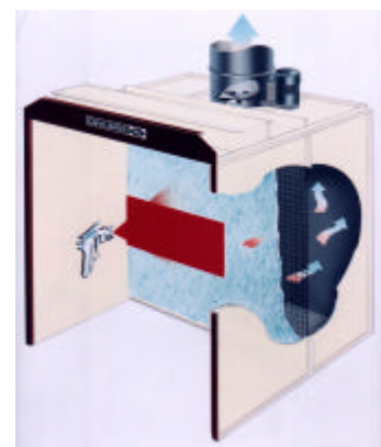
Figure 1.- Dry Filter Type Booth
